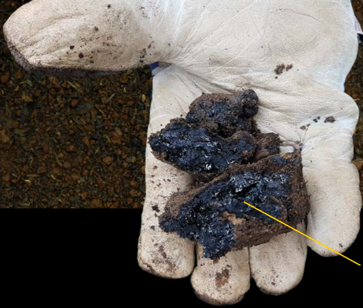
'Blue billy' :) derived from historical gas works. Contains high levels of cyanide and ammonia compounds.
