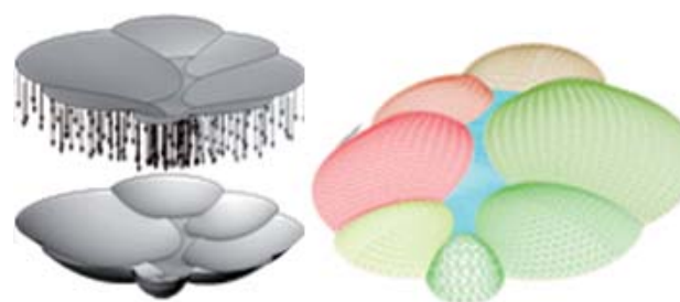
Hanging chain model for Scunthorpe Gridshell
